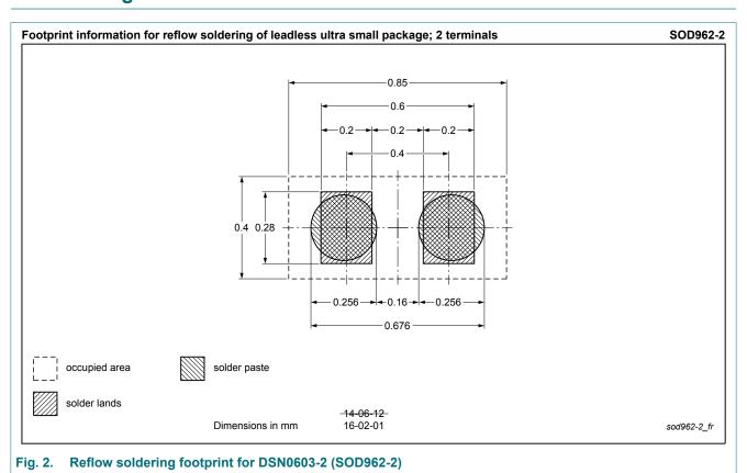
silicon, leadless ultra small package; 2 terminals; 0.4 mm pitch; 0.6 mm x 0.3 mm x 0.3 mm body
