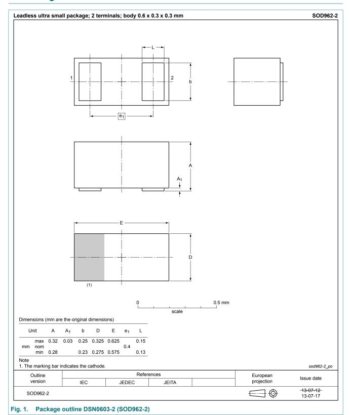
silicon, leadless ultra small package; 2 terminals; 0.4 mm pitch; 0.6 mm x 0.3 mm x 0.3 mm body
